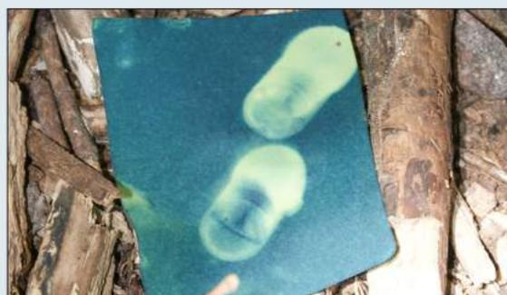
*The horse chestnut contains a water-soluble, UV-active substance between its bark and wood. This chemical substance provides light protection by absorbing UV radiation. The left snap-capped vial contains water as a blank; the right snap-capped vial contains horse chestnut extract. The upper shade in the right picture is more yellow-green due to the sunscreen through absorption of the horse chestnut extract.*
