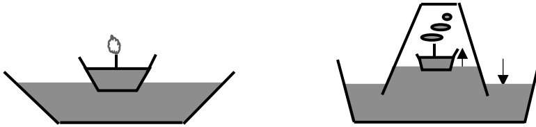
Figure 6: Experiment on the phenomenon of air pressure used in a teacher-training session in CPF
